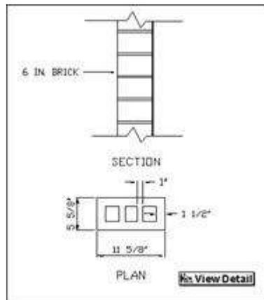
6 IN. BRICK  $w = 130 \text{ lb/ft}^3 \times [(0.60)(5.63 \text{ in.}) / 12 \text{ in./ft}] = 36.6 \text{ lb/ft}^2$
