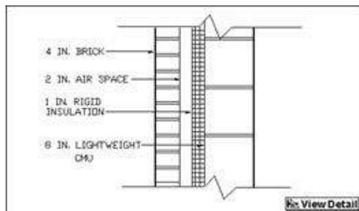
4 IN. BRICK  $HC = 5.9 \text{ Btu/(ft}^2\text{-}^\circ\text{F)}$  (from Fig. 1a)
