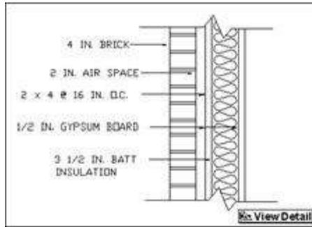
4 IN. BRICK  $w = (130 \text{ lb/ft}^3) \times [(0.75)(3.63 \text{ in.}) / 12 \text{ in./ft}] = 29.5 \text{ lb/ft}^2$
